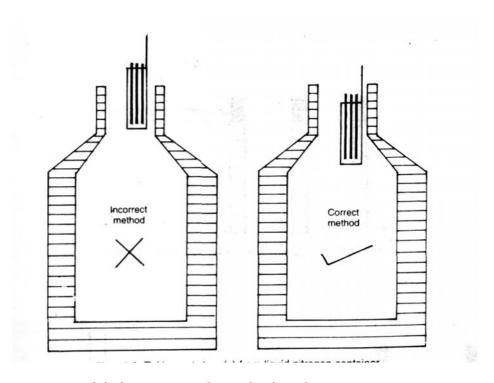
Fig 4 Never lift the canister above the frost line
